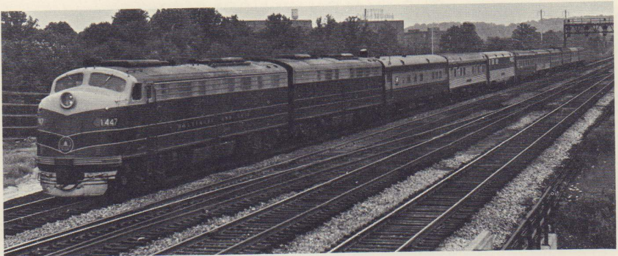
THE CAPITOL LIMITED: Today's Capitol Limited provides first-class passenger service between Washington and Chicago. (Note the cars making up this train. They are from many railroads, illustrating the flexibility engendered by the standardization of rail gauges in 1886.)
